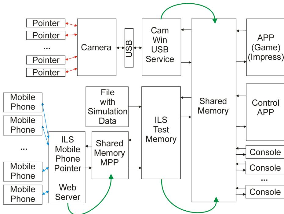
The pointers send out **short invisible light flashes** to the screen which the camera detects (X/Y). Within the light beam also the button states are encoded and in a special case also the pointer unique serial number. The camera can also send commands to the pointers using an **RF transmission (2.4GHz)**. The camera is connected via USB to the PC.
