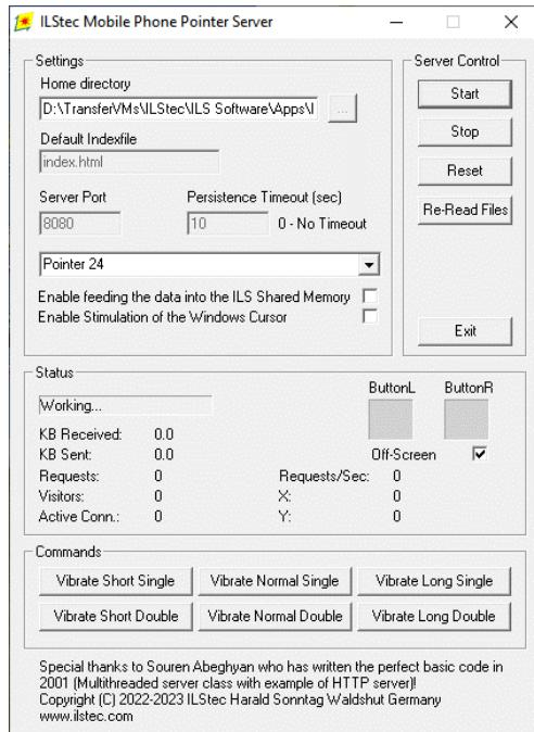
You can select a specific mobile phone (named “Pointer 24” in the above picture), naturally the same number must have been entered on the mobile phone.
